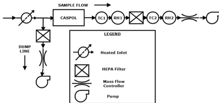
**Figure 1B.** A schematic of the experimental setup of the CASPOL on top of the Moody Tower during DISCOVER-AQ.
