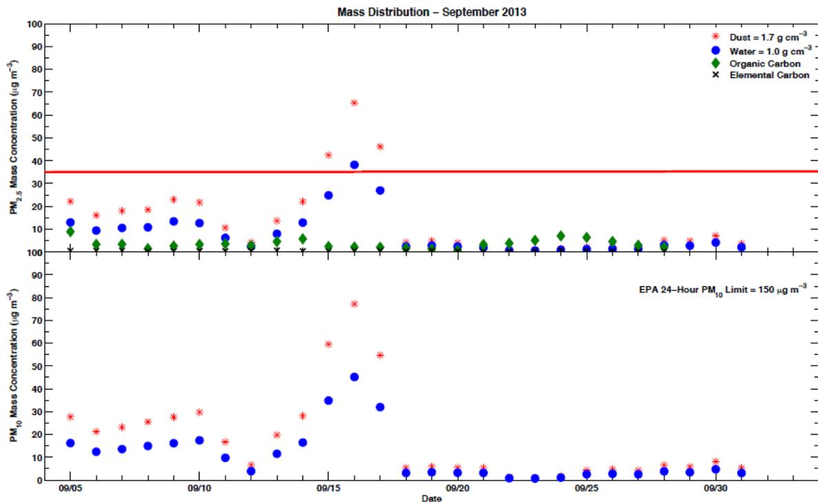
**Figure 4.** The CASPOL estimated daily averaged PM<sub>2.5</sub>, organic carbon, and elemental carbon mass concentrations (top panel) and PM<sub>10</sub> mass concentrations (bottom panel) for the month of September, 2013. The density of dust and water were used as upper and lower bounds of mass respectively. The red bar represents the EPA's PM<sub>2.5</sub> 24-hour average limit.
