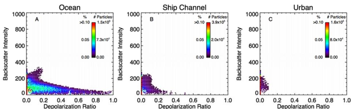
**Figure 2.** The scattering signatures for all of the data in the Ocean, Ship Channel, and Urban sources.
